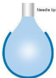
Figure 6: Pendant drop method. The volume (or the weight) of a pendant drop is proportional to the liquid surface tension (Holmberg et al. 2002).
