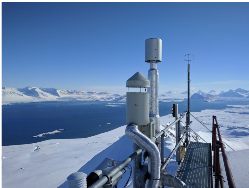
Figure 1: View from Zeppelin station, Svalbard, showing the air inlets used to sample aerosol particles and cloud droplets. Data from this site will be mainly used in this study.
