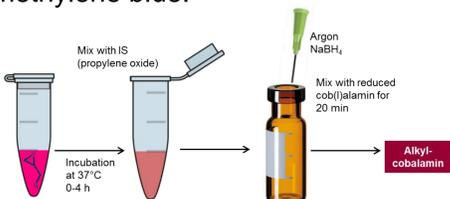
Figure 2. Glycidol stability, measured as cob(I)alamin adducts (alkylcobalamin).
