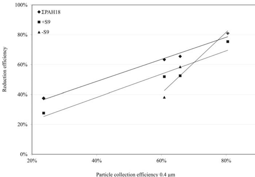
**Fig. 5.** Removal efficiency of  $\Sigma$ PAH18 and reduction of mutagenicity (both +S9 and -S9) downstream of the test objects versus the collection efficiency of 0.4- $\mu$ m particles.
