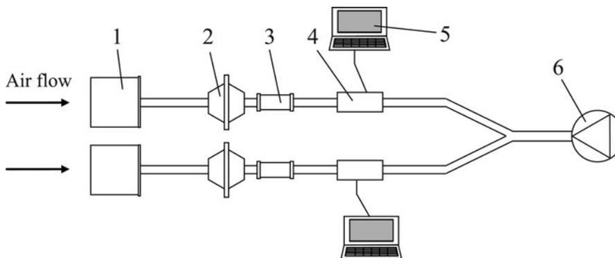
**Fig. 1.** Schematics of the air sampling system depicting: (1) test object holder, (2) sampler holder, (3) PUF holder, (4) airflow/volume measurement device, (5) computer, and (6) high-pressure fan.
