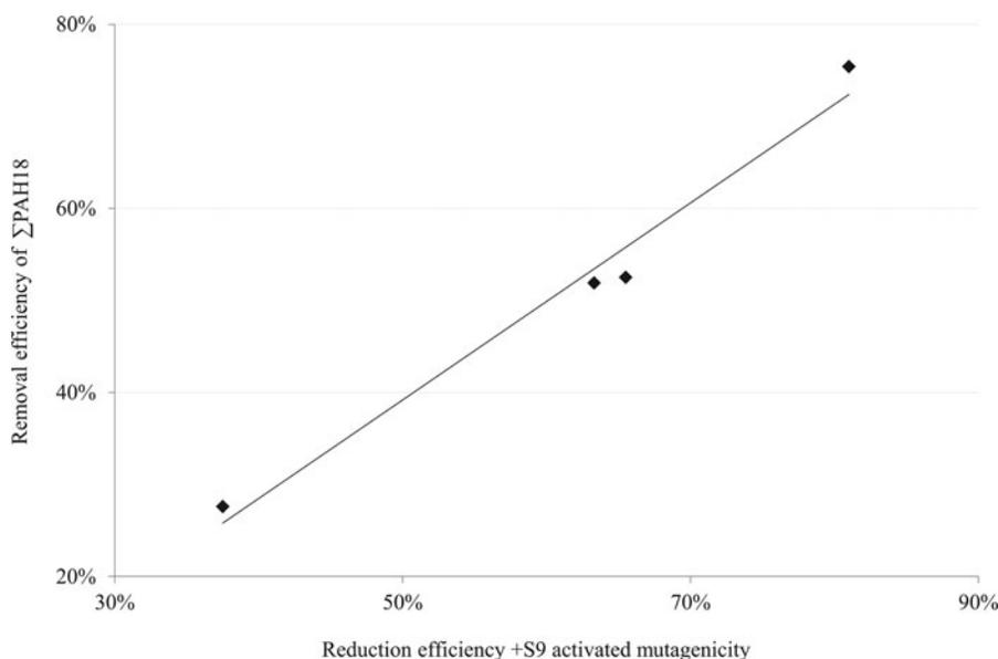
**Fig. 4.** Removal efficiencies of  $\sum\text{PAH18}$  versus the reduction of S9 activated mutagenicity (+S9) for the different test objects.
