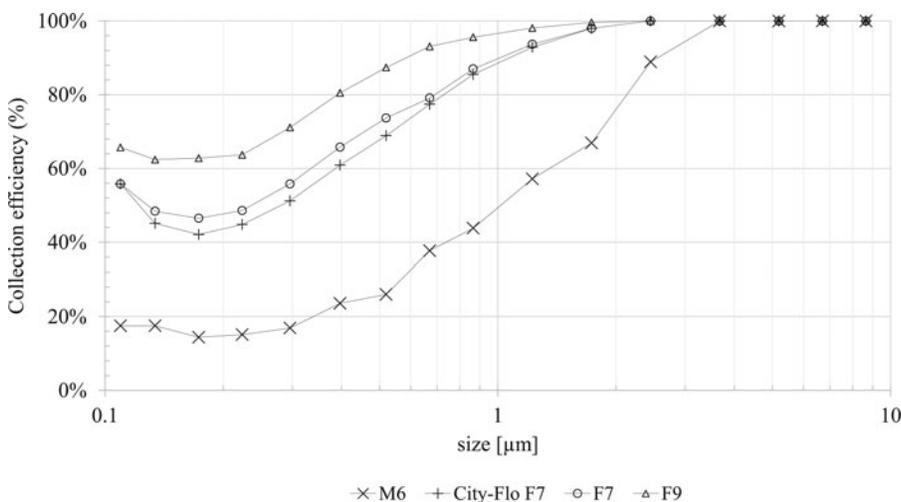
**Fig. 2.** Collection efficiencies of particles in the size range 0.1–10  $\mu$ m for the four different test objects.
